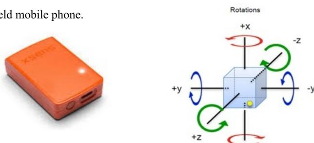
Figure 2. Xsens wireless sensor (left panel) and its 3 dof rotations (right panel).
